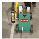
Marking along pallets and walls thanks to its offset arm
